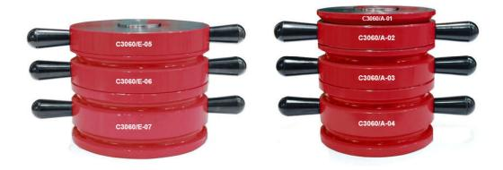
Distance pieces are used to reduce the amount of vertical clearance between the upper platen and the lower platen. 600 to 3000 kN machines are supplied with 205 mm and 165 mm dia distance piece.
